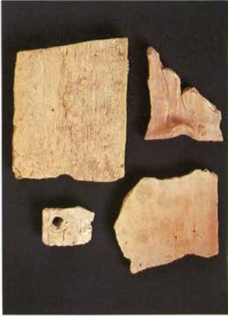
Fragments of roof tiles used on Government House from about 1788–89 to 1794. Made locally and attached to the roof by wooden pegs, they tended to collect water and become very heavy. They were replaced by wooden shingles.
